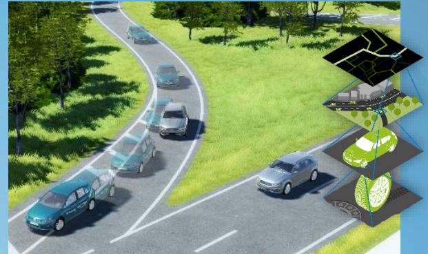
Simulation of a driving manoeuvre in a virtual test field. The simulation takes place on different abstraction levels (traffic flow, vehicle guidance, driving physics, etc.).
